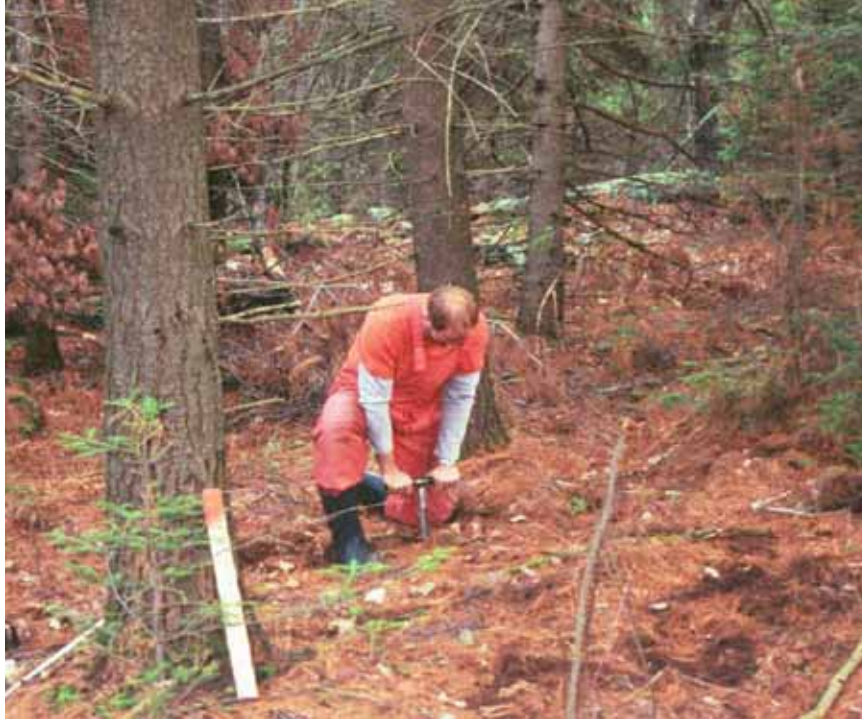
Figure 7: Collection of a soil parent material sample with Dutch augur.
